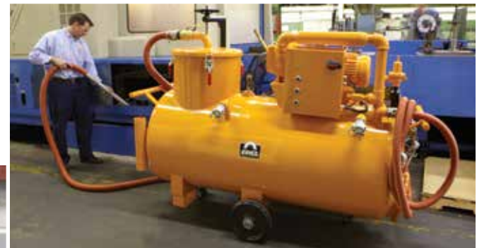
Machine tool coolant, chips and sludge are easily vacuumed out of the sump.
